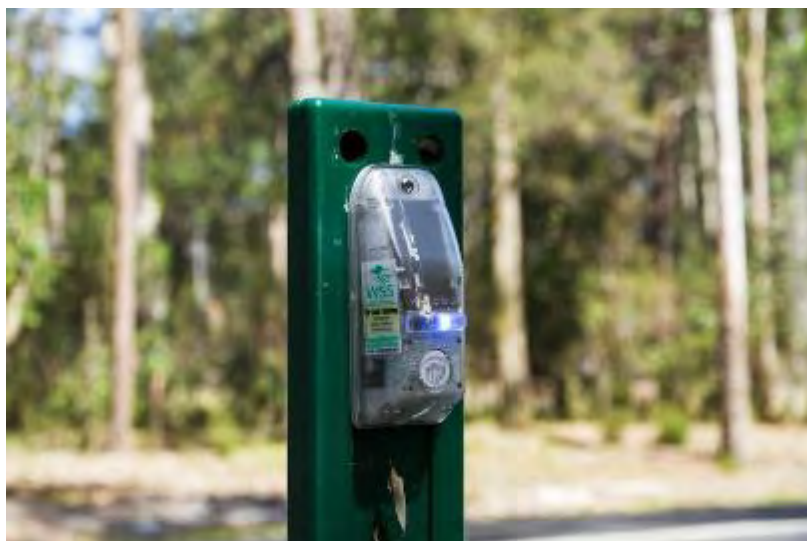
Figure B.6.8 Eurobodalla Shire Council's virtual fence trial consisting of electronic devices attached to roadside posts
