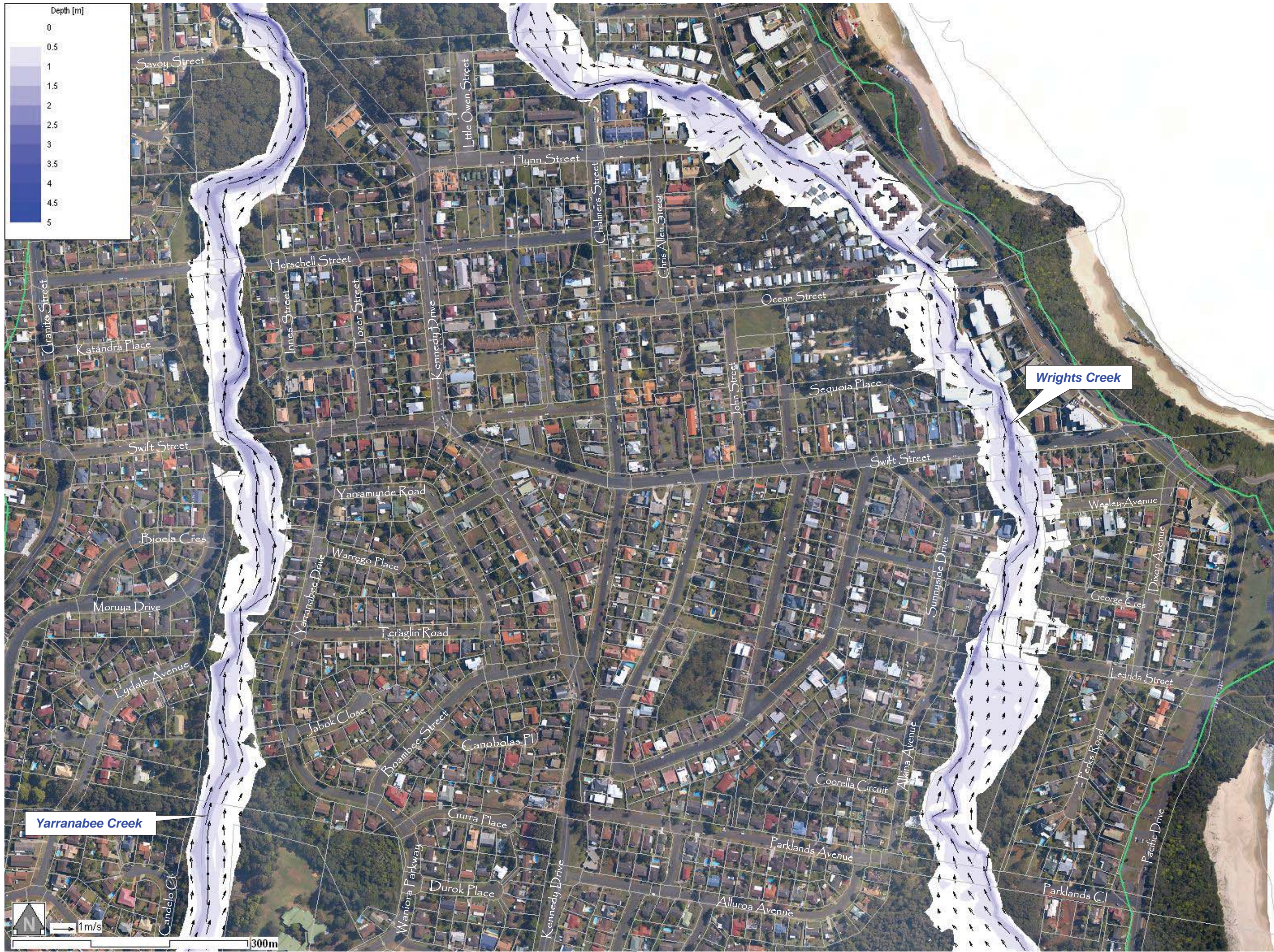
FLOODWATER DEPTHS AND VELOCITIES ALONG THE CENTRAL REACHES OF WRIGHTS CREEK AT THE PEAK OF THE 100 YEAR RECURRENCE FLOOD
